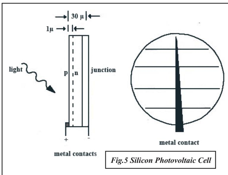
Fig.5 Silicon Photovoltaic Cell
