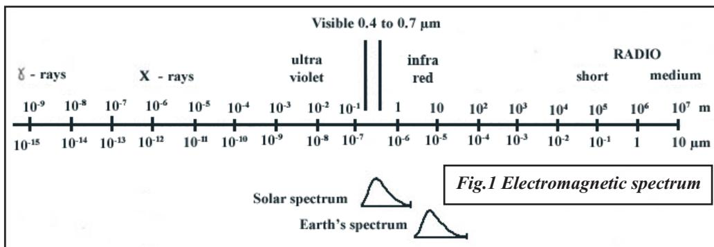
Sun light contains wavelengths over a continuous spectrum with maximum energy lying between 0.3  $\mu\text{m}$  and 1.5  $\mu\text{m}$ , see Fig 1.
