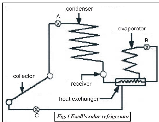
**Fig.4 Exell's solar refrigerator**
